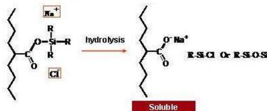
The hydrolysis rate is controlled and therefore a stable erosion rate is obtained leading to a steady release of biocides. Since the silyl groups have no biocidal function, the presence of biocides is still required. Transocean Armada is compatible with standard Transocean Anticorrosive schemes and can be used to upgrade existing Cleanship systems.
