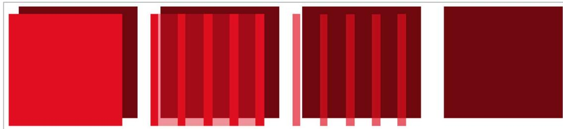
Figure 6: polishing pattern over time, visible higher DFT in spray overlaps while the first coat reduces in thickness
