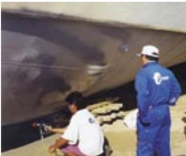
The gelcoat should be degreased thoroughly with Transocean Gelclean to eliminate traces of wax, paraffin and other contaminants. High-pressure wash with fresh water and allow thorough drying. Disc abrade to an even, matt finish. Remove dust and debris prior to painting.
