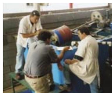
Rotor machine to measure erosion properties
