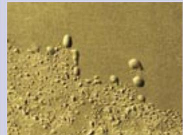
However, not all bubbles are the result of osmosis. If the blisters are filled with liquid and have an acidic smell, osmosis is very likely. In case blisters do not contain fluids but are the result of air bubbles, repairing is relatively easy by just sanding and priming.
