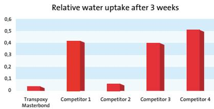
Relative water absorption by the coating. Low values indicate better corrosion protection. Again, Transpoxy Masterbond has the lowest values of all tested surface tolerant epoxies.
