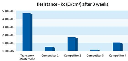
Resistance (Rc) in Ω/cm² offered by the coating. Higher values mean better corrosion resistance. Transpoxy Masterbond offers the highest resistance value.
