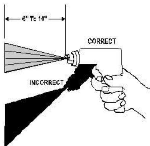
Hold the gun perpendicular to surface being sprayed
