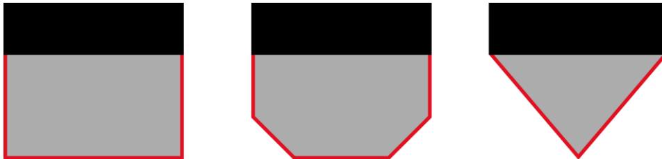
Figure 7: sectional shapes; box (set as 100%), shaped hull ( \pm 88\% vs box), triangle ( \pm 71\% vs. box)
