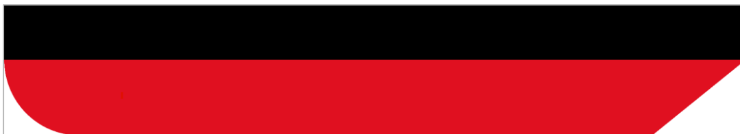
Figure 5: long hull, short bow shape, correction factor \approx 90\% vs. rectangular shape
