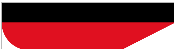
Figure 6: shorter hull, longer bow shape, correction factor \approx 80\% vs. rectangular shape
